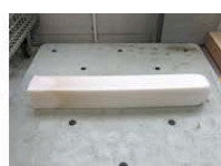
Materials like polystyrene are melted in a melting machine at the recycling center, then cooled and formed into ingots.
