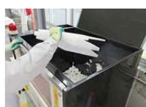
Materials like polystyrene are melted in a melting machine at the recycling center, then cooled and formed into ingots.
