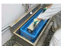
Materials like polystyrene are melted in a melting machine at the recycling center, then cooled and formed into ingots.
